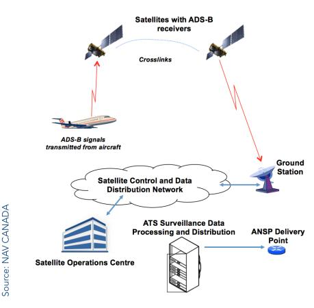
Figure 3 - Space-Based ADS-B Concept
